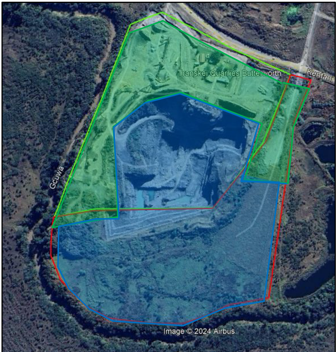
Figure 6: Satellite image of the mining area to be rehabilitated upon closure. The mining and processing related areas (green) will revert to agricultural/residential use upon rehabilitation, and the quarry pit (blue) will be rendered safe and left as a landscape feature. (Image obtained from Google Earth)
